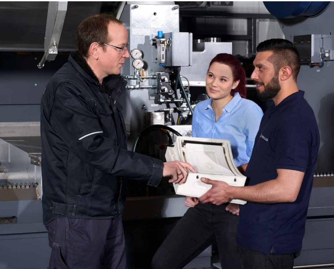
Time-saver: the steady rest pads produced with the 3D printer can be changed manually
