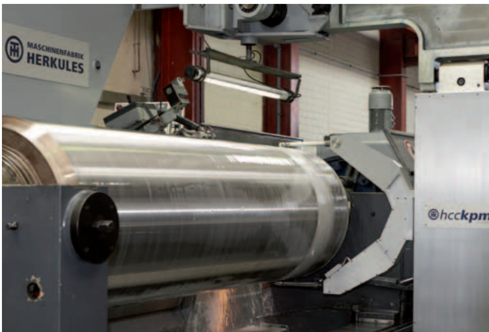
The HCC/KPM system and its two measuring sensors allow simultaneous measuring and processing of events during grinding.
