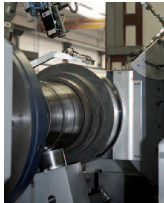
A protective hood covers the grinding wheel
