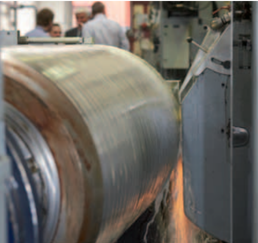
Protective hood for CBN grinding
