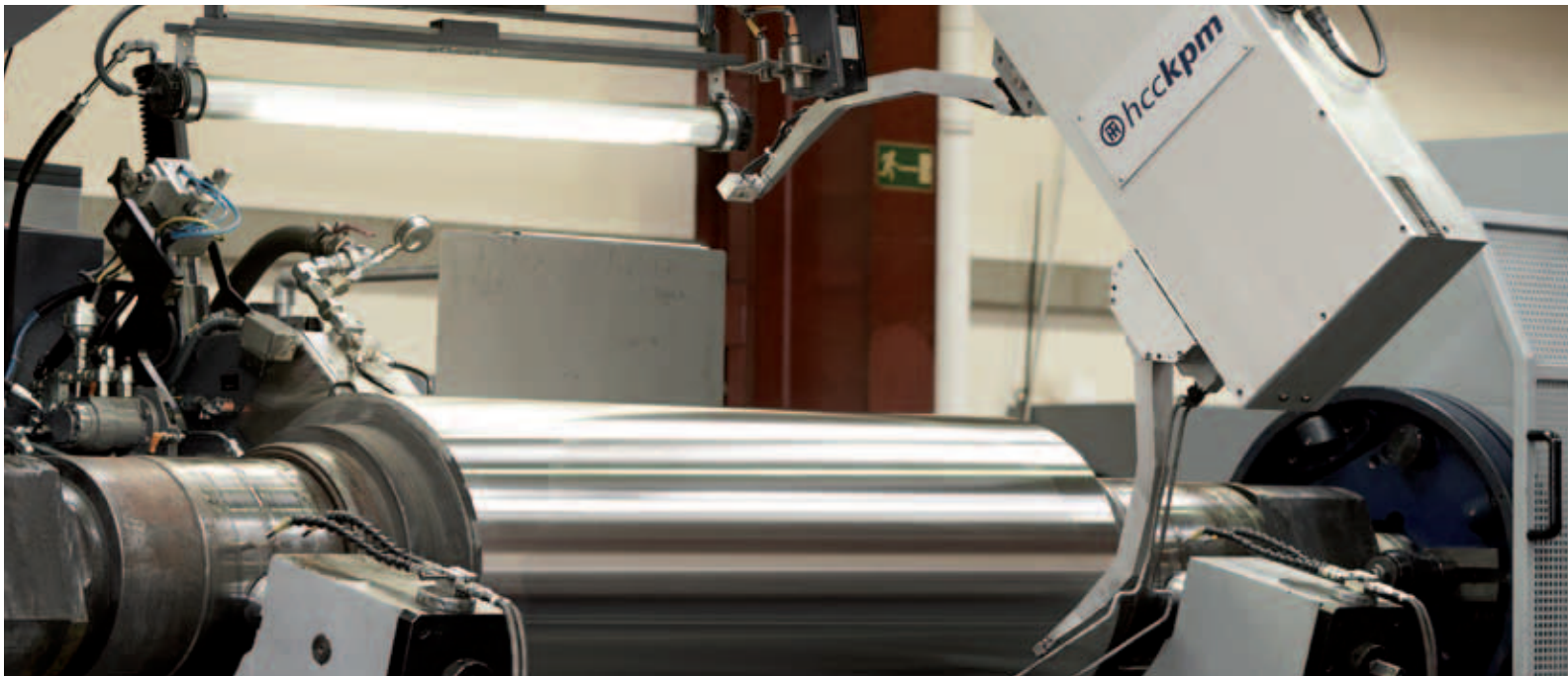
Reproducible results in finish grinding with CBN coating – the innovative technology package by Herkules and MACH ROTEC
