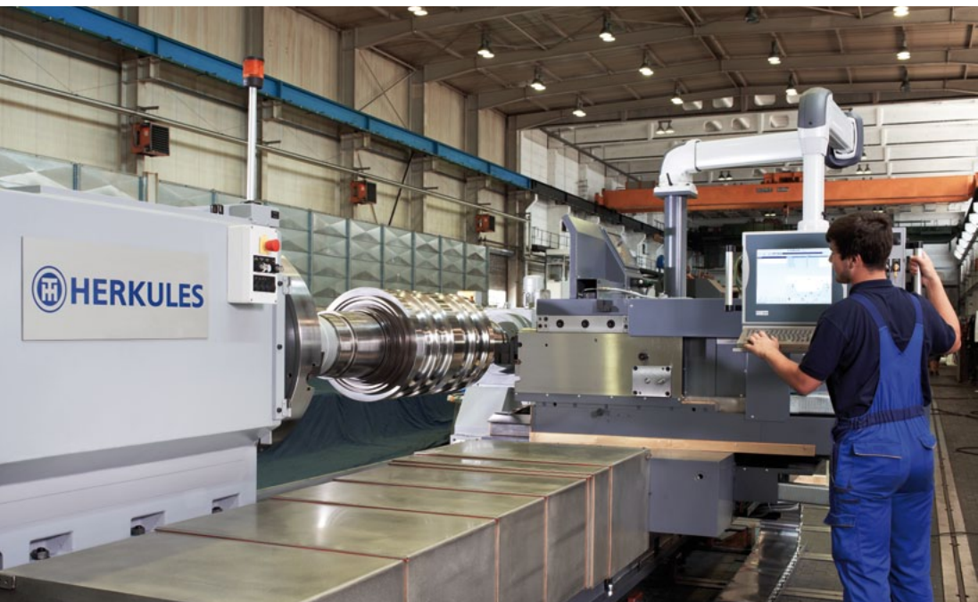
Newly developed heavy duty lathe P 500 Power for Badische Stahlwerke GmbH
