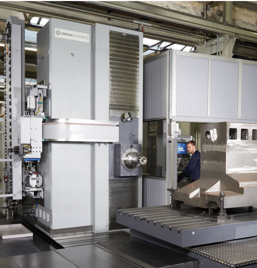
New, high precision horizontal boring mill from UnionChemnitz at Herkules in Siegen.
