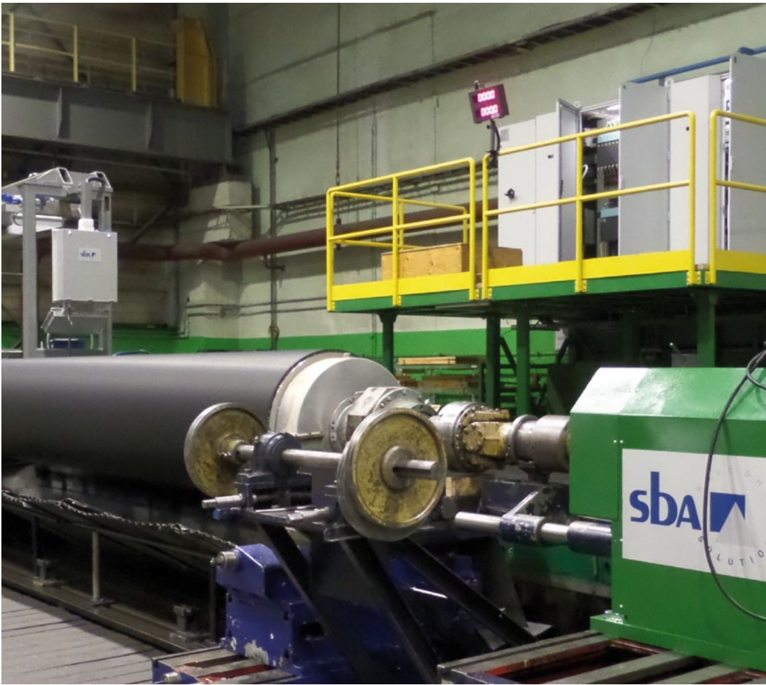
Dronsfield roll grinder for the paper industry, modernized by SBA
