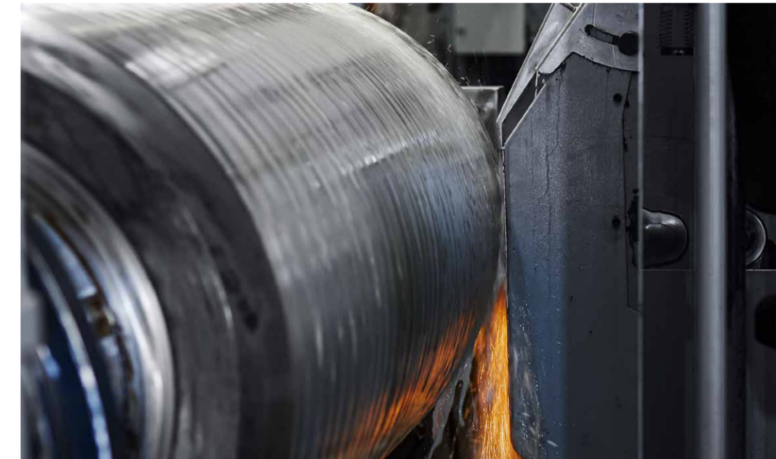
Herkules MACHtechnology is a pioneer in roll grinding with CBN wheels
