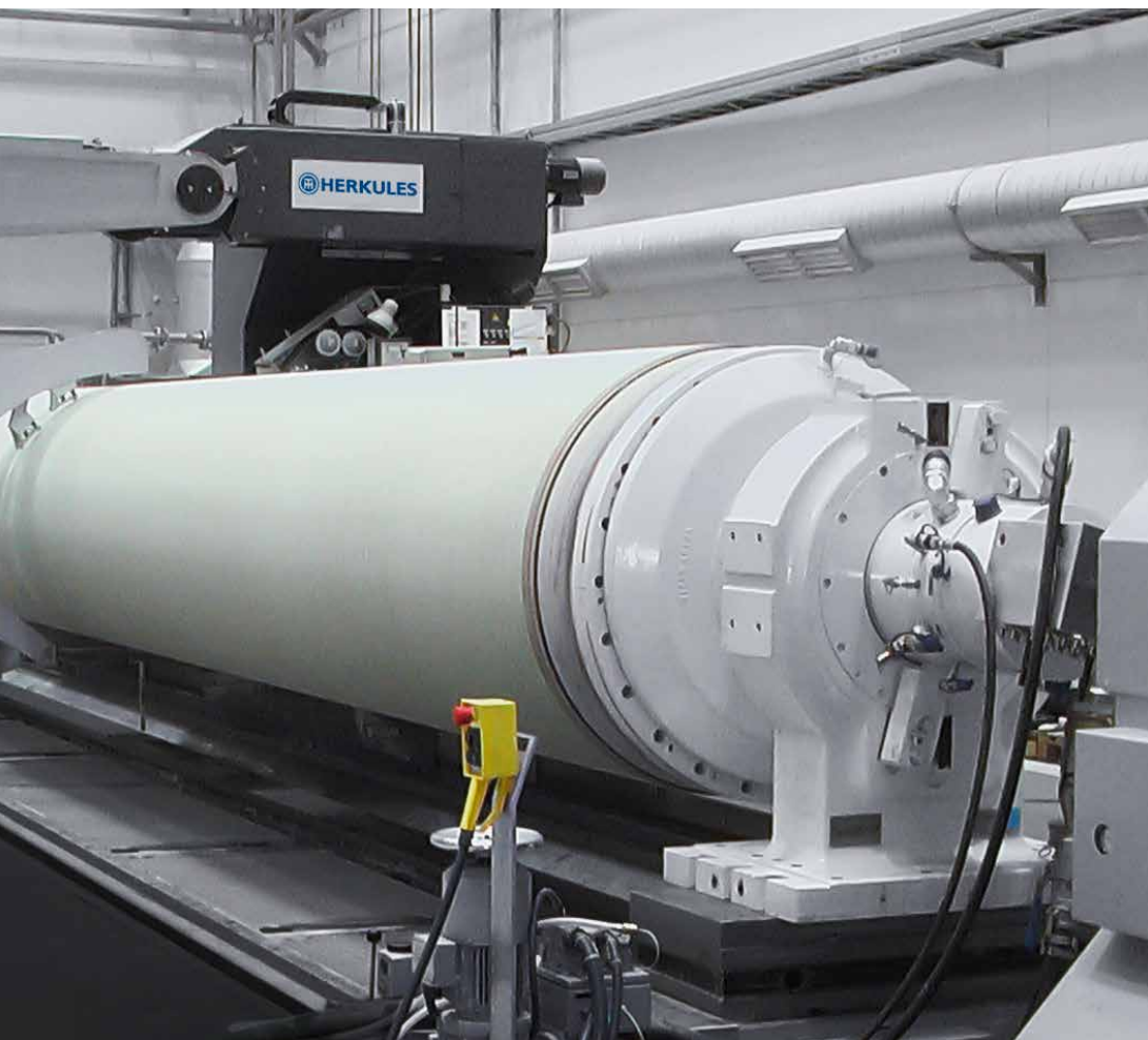
Herkules roll grinders machine paper rolls up to 17.5 m in length and 2.5 m in diameter
