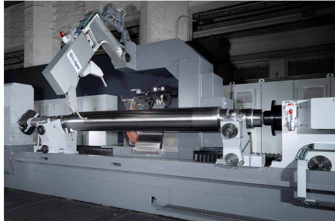
The WS 450 is equipped with precise measuring systems such as the C-Frame Caliper
