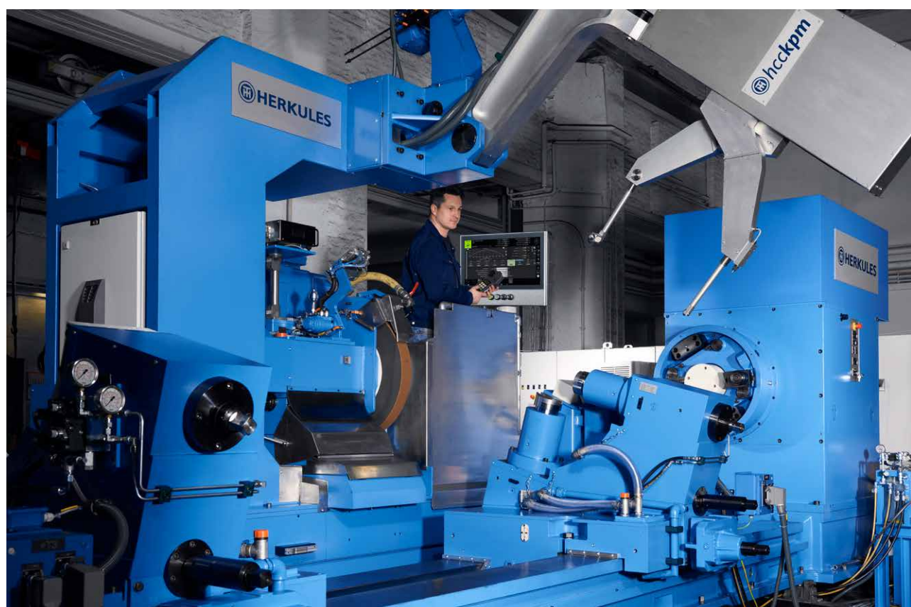
At the end of the C-frame, different sensors ensure perfect inspection of the roll
